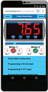
PD8-765 operators can take advantage of the Trident Virtual Meter. This is a great tool for getting comfortable with programming 4-20 mA, 0-10 V, Thermocouple and RTD inputs. You can also practice scaling the meter without a signal, calibrating the meter, setting up relays, and more. The Trident Virtual Meter is available on your desktop or mobile device. Just visit [TridentVirtualMeter.com](http://TridentVirtualMeter.com) to start practice programming your PD8-765 meter.
