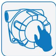
The ProtEX-MAX PD8-765 is equipped with four sensors that operate as through-glass buttons so that it can be programmed and operated without removing the cover (and exposing the electronics) in a hazardous area. The SafeTouch buttons are configured by default to duplicate the function of the front panel mechanical pushbuttons associated with the integrated meter.
