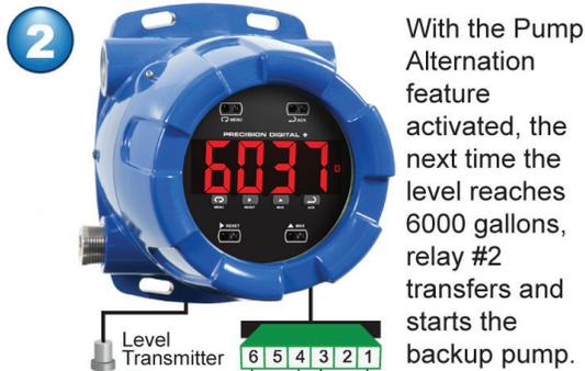
With the Pump Alternation feature activated, the next time the level reaches 6000 gallons, relay #2 transfers and starts the backup pump.
