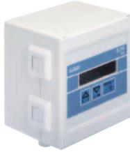
The device is equipped with a 4...20 mA current output (analogue output), a digital output (pulse output) and two totalizers. Some versions are also fitted with two relay outputs. The device operates on a 2- or 3-wire system and needs a 12...36 V DC or a 115/230 V AC power supply.
