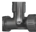
When liquid flows through the pipe, the paddle wheel with 4 inserted magnets is set in rotation, producing a measuring signal in the sensor (Coil or Hall sensor). The frequency modulated induced voltage is proportional to the flow velocity of the fluid.
