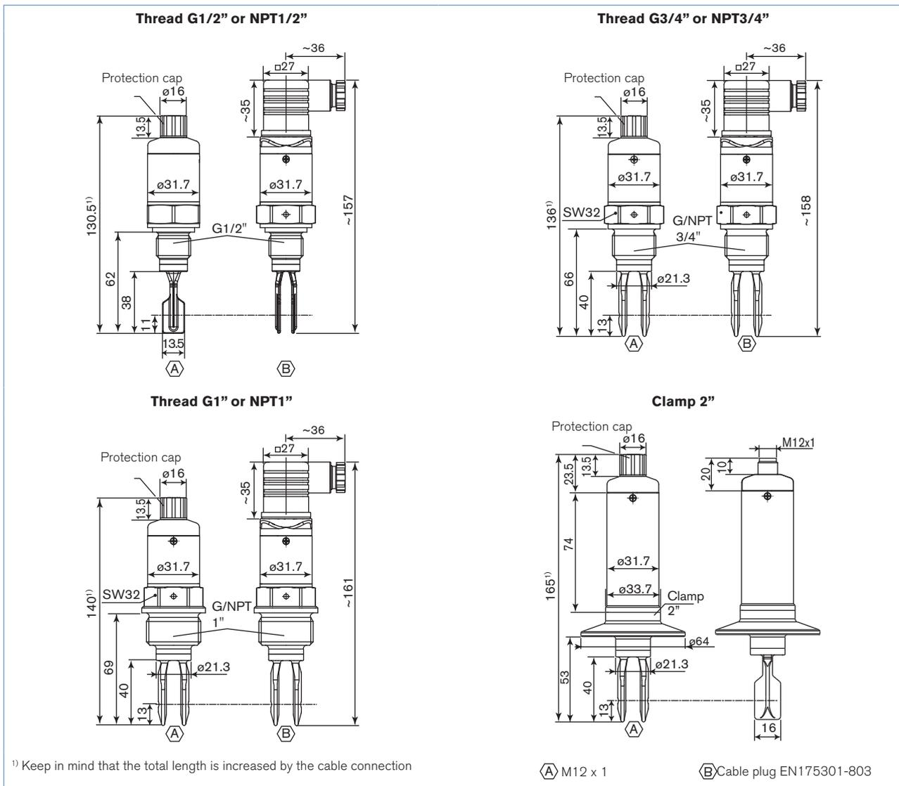
**Ordering chart for the vibrating level switch Type 8110**
