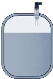
Chemicals are required for sewage water treatment. They are used for precipitation. Phosphate and nitrate are sedimented and separated. For the sludge treatment and neutralization, acids and solvents are stored apart from lime water and ferric chloride. These substances are subject to the regulations for water-endangering substances. Therefore overflow protection systems must be mounted on storage tanks.
