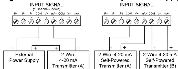
**Figure 6. Transmitter Powered by Ext. Supply or Self-Powered**
