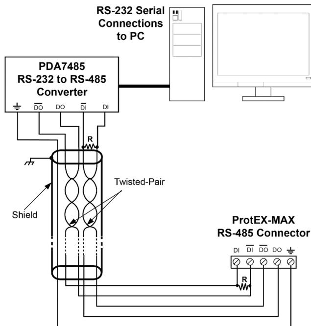
Figure 10: RS-485 Wiring
