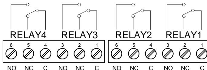
**Figure 12. Relay Connections**
