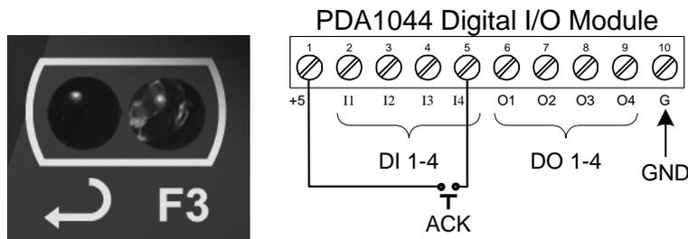
**Figure 19. Acknowledge Relays w/Function Key or Digital Input**
