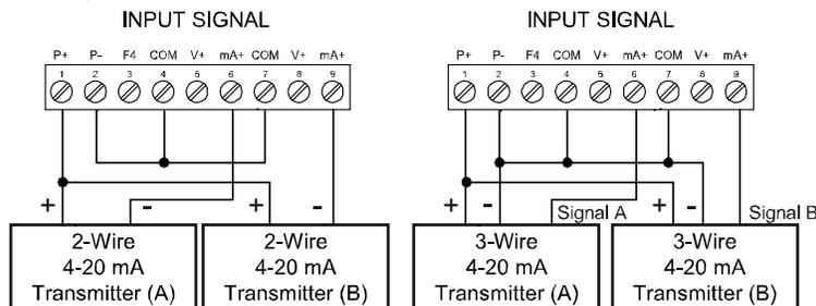
**Figure 5. Transmitters Powered by Internal Supply**
