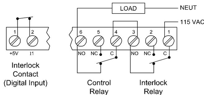
Figure 17. Interlock Connections
