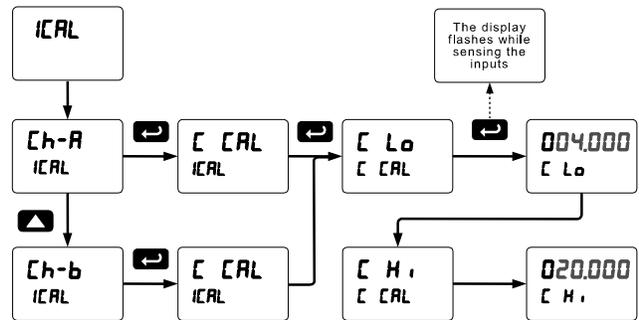
The graphic above shows the calibration of the current input. The voltage input is calibrated in a similar way.
