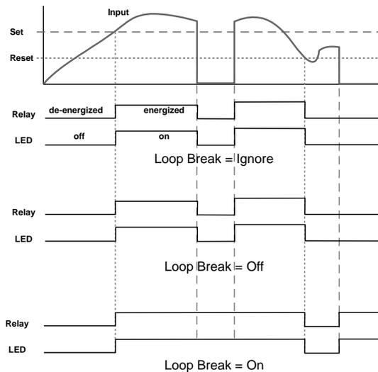
When the meter detects a break in the 4-20 mA loop, the relay will go to one of the following selected actions:
