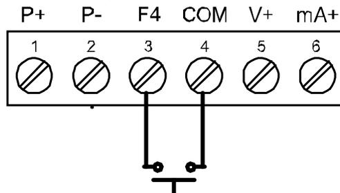
**Figure 20. F4 Digital Input Connections**
