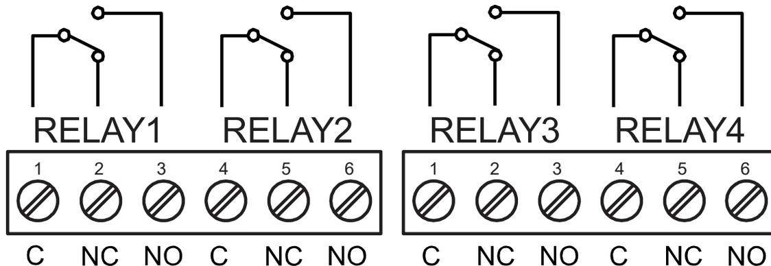
**Figure 12. Relay Connections**
