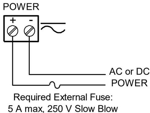
**Figure 8. Power Connections**
