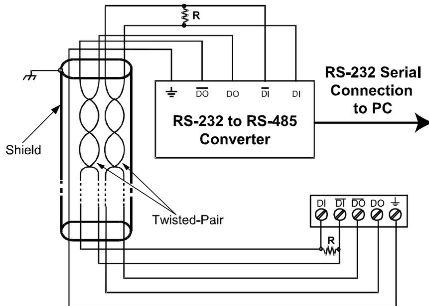
Figure 15. RS-422 or RS-485 Wiring
