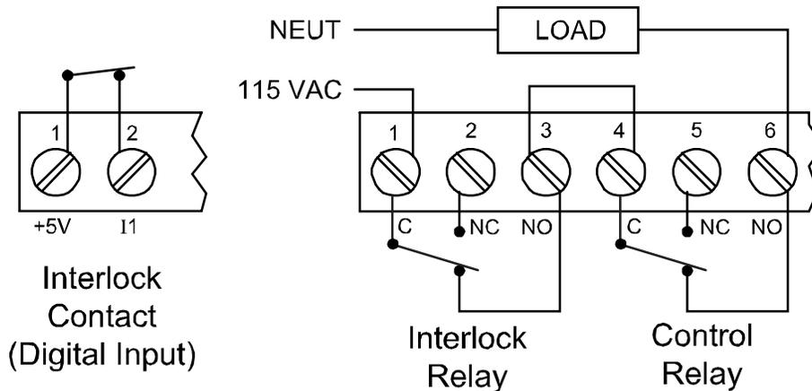
Figure 22. Interlock Connections
