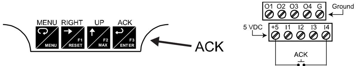
**Figure 23. Acknowledge Relays w/Function Key or Digital Input**
