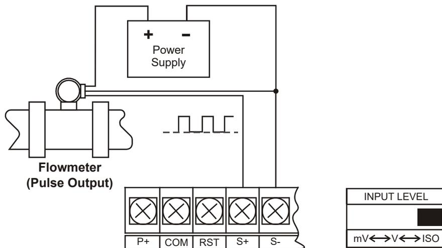
Figure 9: Isolated Flowmeter Powered by External Supply (ISO)
