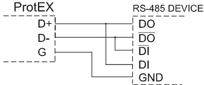
Figure 3: RS-485 Five-Wire Serial Connections
