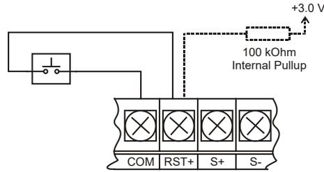
Figure 5: Reset Connections
