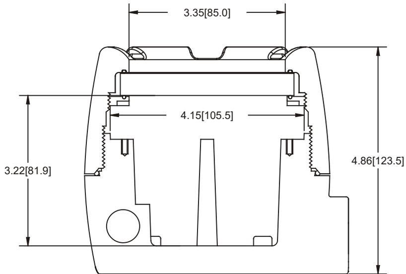
**Figure 17: Enclosure Dimensions – Side Cross Section View**
