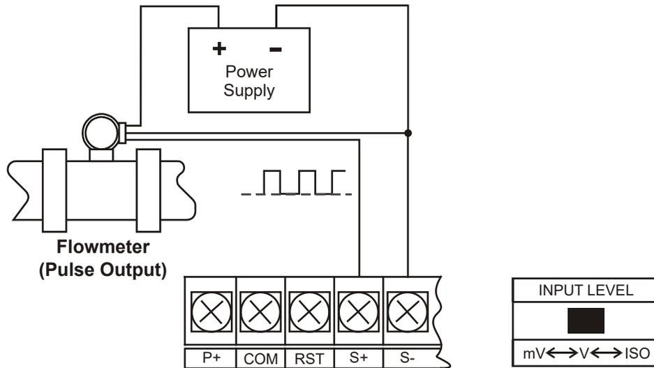
Figure 8: Flowmeter Powered by External Supply (Active)
