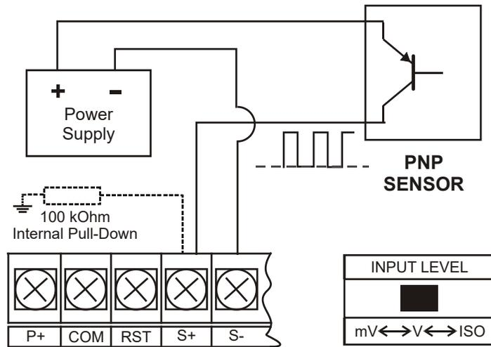
Figure 12: PNP Sensor with External Power (PNP)
