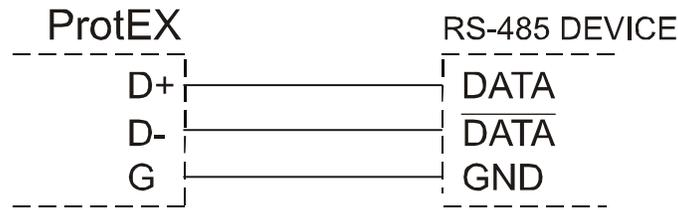
Figure 2: RS-485 Three-Wire Serial Connections
