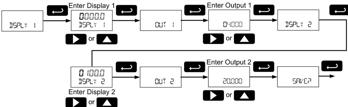
The following diagram details setting the analog output when the source is configured to display on the top display of a feet and inches display model.
