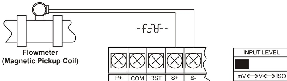
Figure 10: Self-Powered Magnetic Pickup Coil Flowmeter (Coil)
