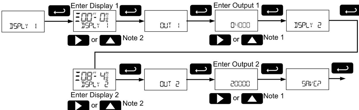
The following diagram details setting the analog output when the source is configured to display on the bottom display.
