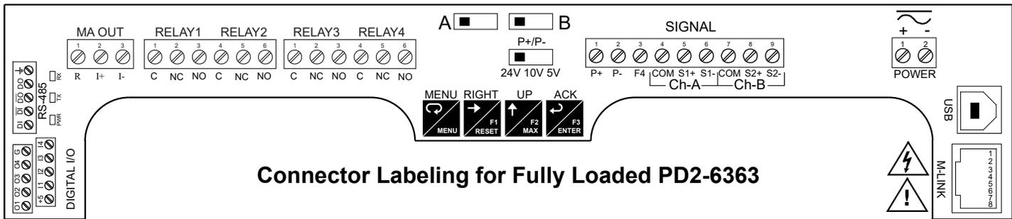
Connector Labeling for Fully Loaded PD2-6363
