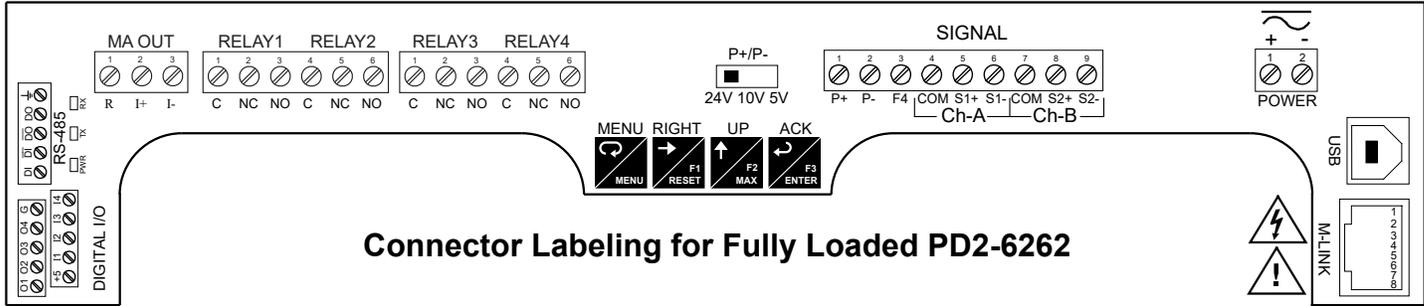
Connector Labeling for Fully Loaded PD2-6262
