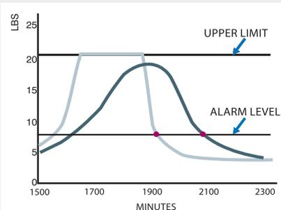
A read out comparison of the SS2000e (left curve) and a slower sensor demonstrates how eliminating long dry-downs can drastically reduce costly shutdown times. In this example, the alarm state is erroneously extended for hours.
