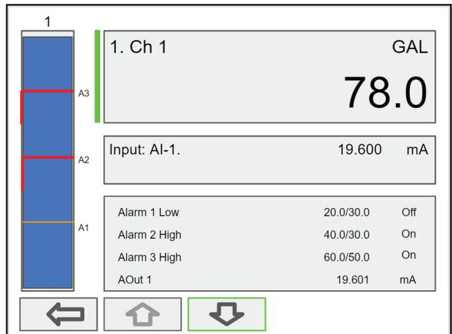
**Active High Alarm:** Indicated by red horizontal and vertical lines. The bottom of the vertical line is the reset point of the high alarm. The high alarm is indicated on the left side of the bargraph.
