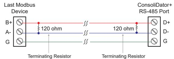
Figure 13. Serial Connections
