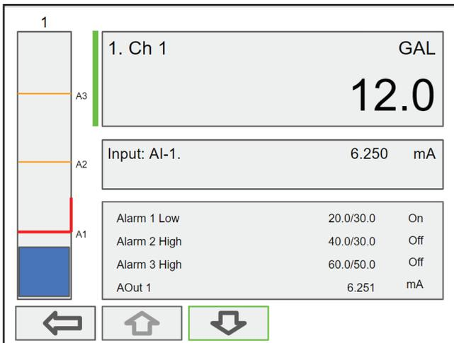
**Active Low Alarm:** Indicated by red horizontal and vertical lines. The top of the vertical line is the reset point of the low alarm. The low alarm is indicated on the right side of the bargraph.
