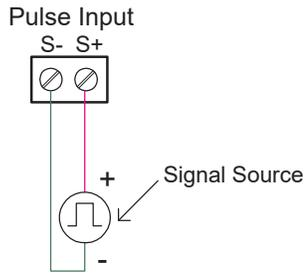
Figure 5. Flow Meter Pulse Input Connections
