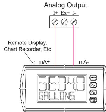
Figure 7. Active 4-20 mA Output Powered by ConsoliDator+
