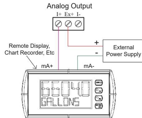
Figure 8. Passive 4-20 mA Output Powered by External Supply
