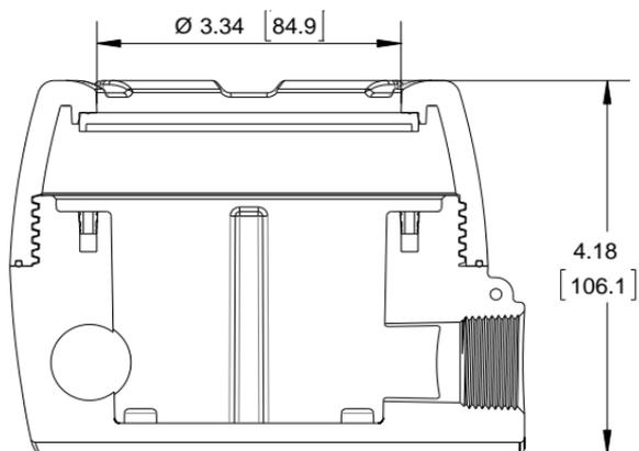
Figure 11. Enclosure Dimensions – Side Cross Section View
