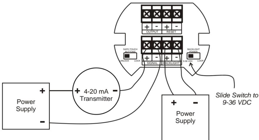
**Figure 4. Input Connections with Externally-Powered Backlight**
