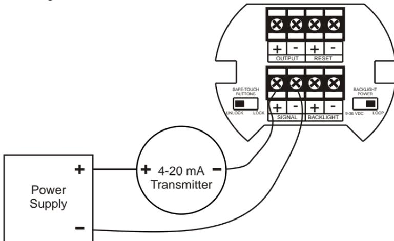
Figure 2. Input Connections without Backlight
