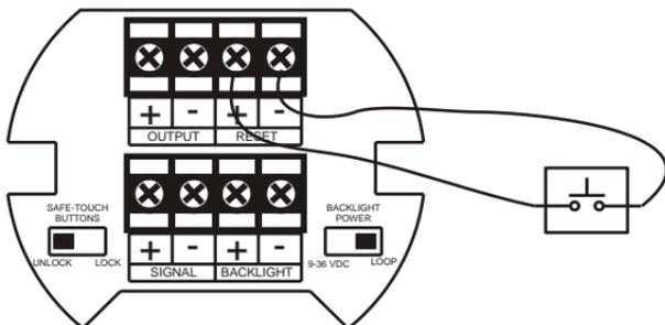
**Figure 5. Reset Connections**
