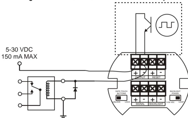
Figure 7. Output Connections
