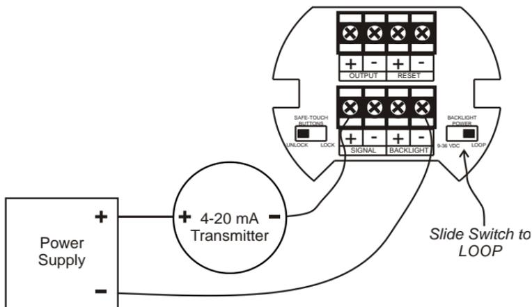
Figure 3. Input Connections with Loop-Powered Backlight
