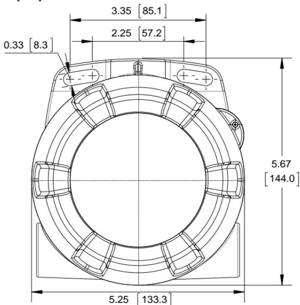
Figure 10. Enclosure Dimensions – Front View
