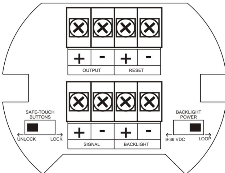
Figure 1. Connector Board
