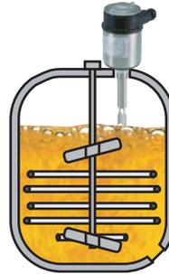
Thanks to the manifold application possibilities, the Type 8112 vibrating level switch is ideal for all applications concerning stock-keeping of liquids.
