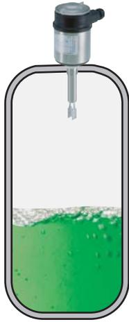
Beside the continuous level measurement, level detection is a main safety characteristic for storage tanks.
